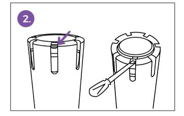
Find the small slot on the top of the thermostatic head. Using the supplied tool, place it into the slot and lift the cap off. You should now be able to pull the shroud off of the thermostatic head.
