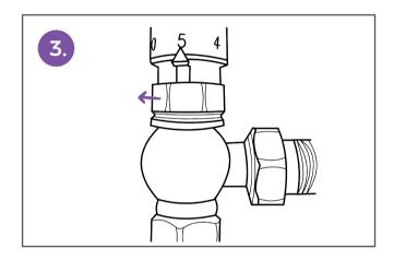
Set thermostat to position 5 and align square over the body. Screw the retaining nut in a clockwise direction until tight. Take care not to overtighten.
