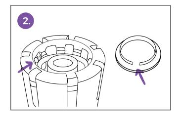
Place the small cap back onto the top end of the thermostatic head. Ensure the small notch is aimed at the small bulge and press until you hear a click.
