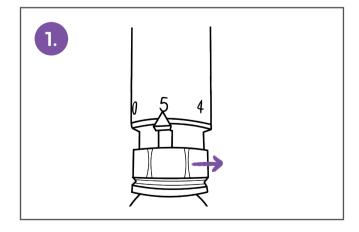
Set thermostat to position 5, unscrew anti-clockwise and remove the thermostatic valve head from the valve body.
