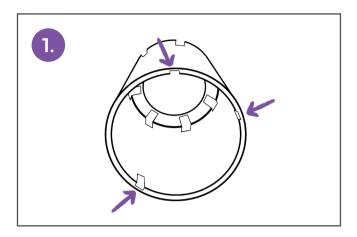
Align the 3 recesses at the bottom end of the shroud with the 3 bulges at the bottom end of the thermostatic head. Push the shroud down onto the head until you hear a click.
